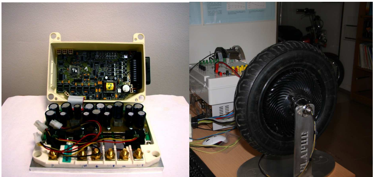
Fig: Production ready ECU with power stage (left) and in-wheel PMSM drive (right)
