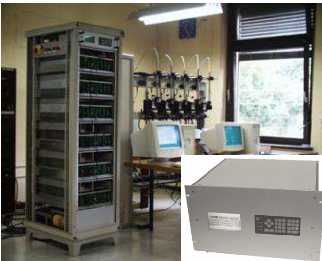
Fig: Stationary and portable version of three phase power source
